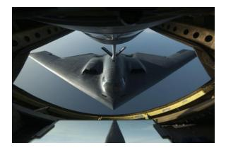
Eventually, it's time to refuel. The B-2s meets KC-135 Stratotankers at least twice on the way to Libya. It's a coordinated dance that must occur no matter what the weather or time of day. The airplane in need of fuel flies directly behind the tanker. The tanker then extends a telescoping fueling boom. The end of the boom—the fuel nozzle—latches into a small hole in the receiving aircraft, and the fuel pumps as the conjoined aircraft fly in harmony.
