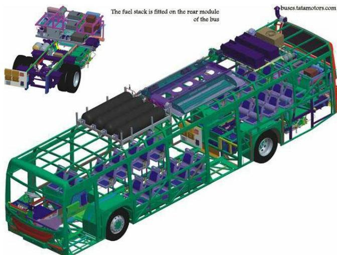
This electricity is used to charge the battery to power the motor of the bus. A number of fuel cells are combined to form a fuel cell stack, which is placed in the rear module of the bus.
