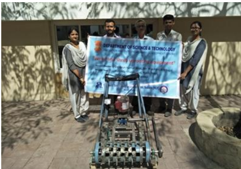
Weed, shrub uprooting machine: Uproots the unwanted plants from roots
